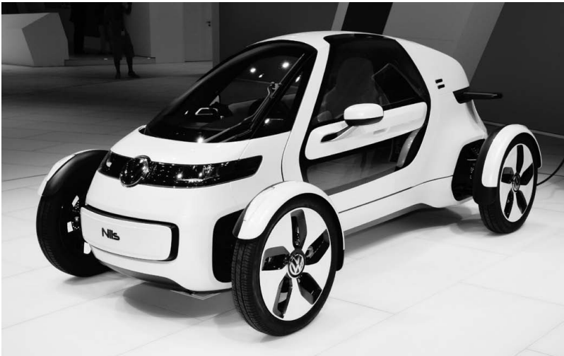
VW NILS: 3040×1390×1200mm, 460kg, Max 130km/h, Cruising Range 65km
