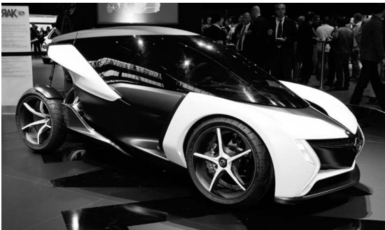
Opel RAK e: L3000×H1190mm, 350kg, EV, Cruising Range 120km
